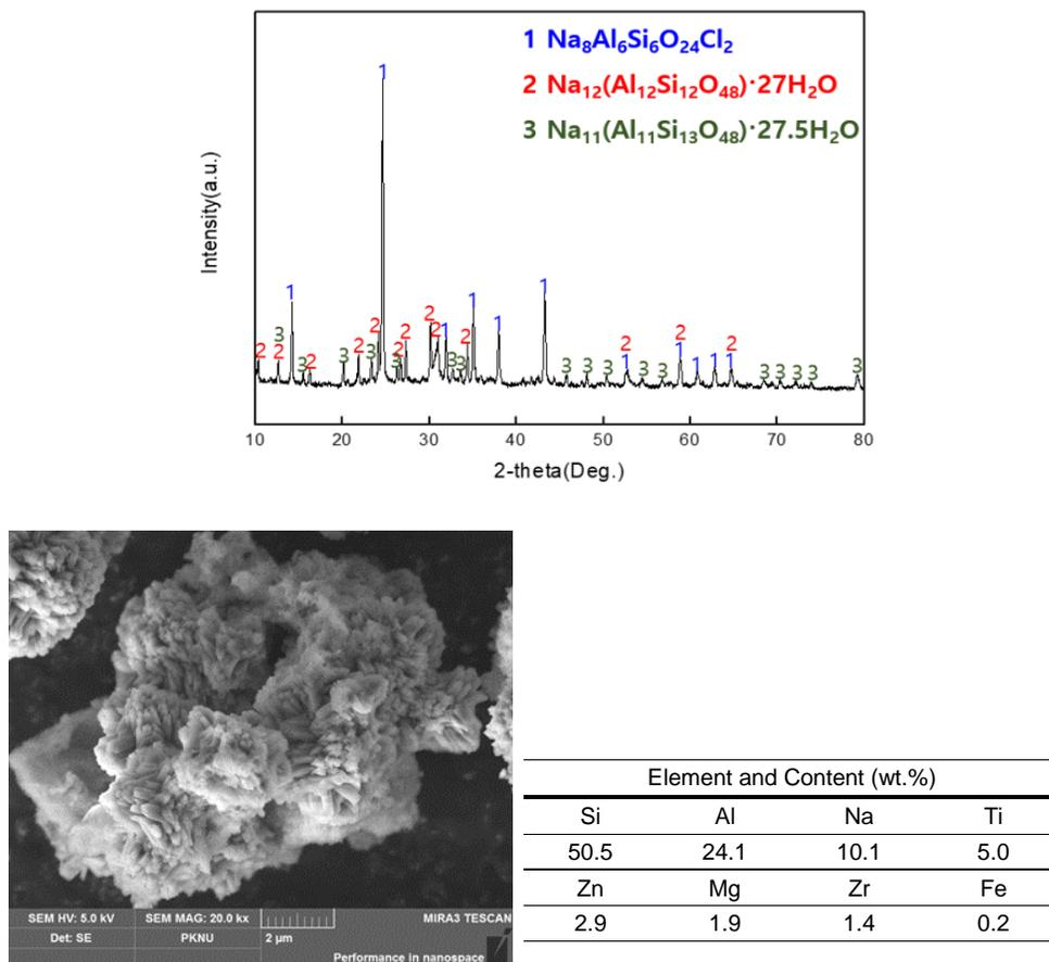
Figure 5: Analysis results of lithium-removed zeolite LAS.
