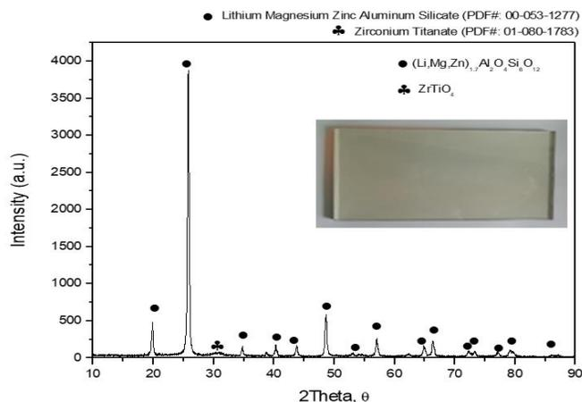
**Figure 1:** Raw LAS sample (top) and XRD analysis results of the raw LAS sample (bottom)
