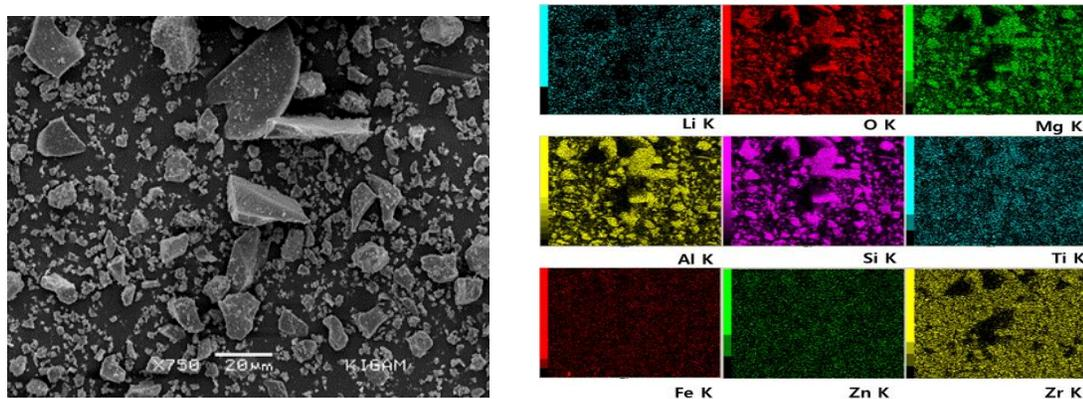
**Figure 2:** SEM analysis of the raw LAS sample (left) and mapping analysis results of the raw LAS sample (right).
