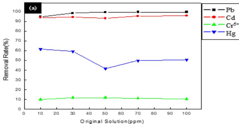
**Figure 8.** The influence of initial heavy metal solution on heavy metal removal rates (a) Li-removed zeolite, (b) K-zeolite
