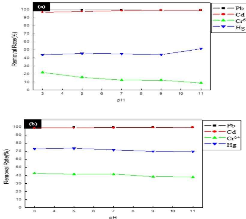
Figure 9: Effect of pH on heavy metal removal rate (a) Li-removed zeolite, (b) K-zeolite.
