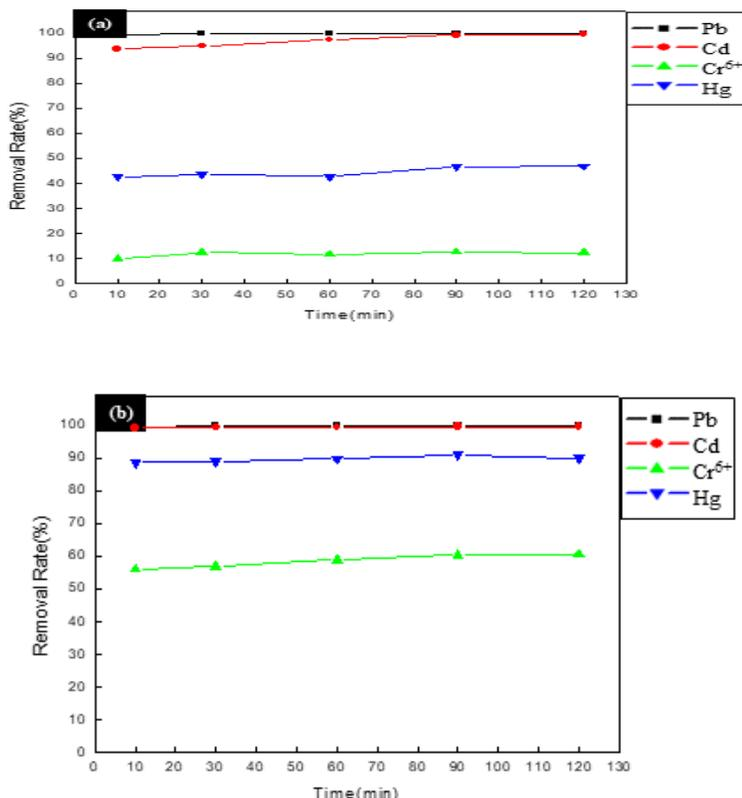
**Figure 7:** Effect of pH on heavy metal removal rate (a) Li-removed zeolite, (b) K-zeolite.
