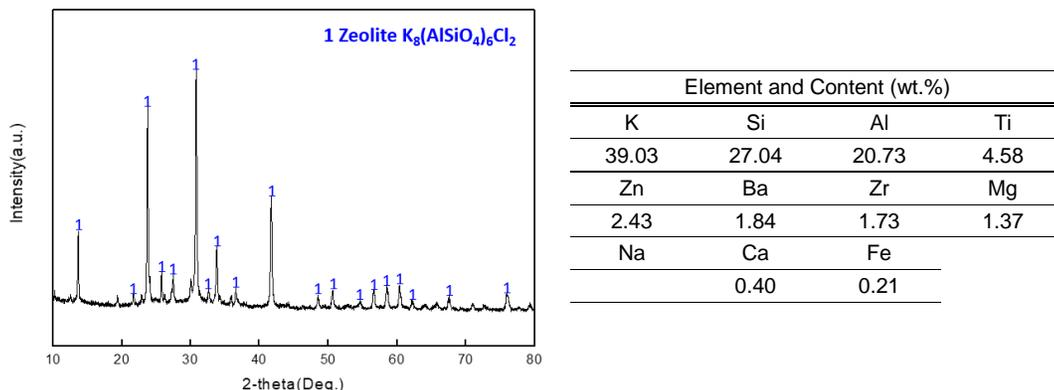
**Figure 6:** XRD/XRF results of KCl-modified Na-zeolite experiment.
