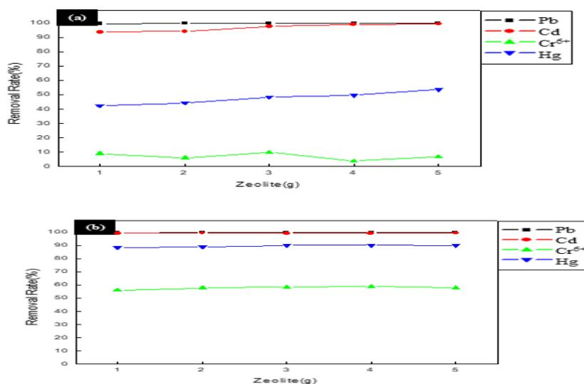
**Figure 6:** Influence of Zeolite Addition Amount on Heavy Metal Removal Rate (a) Li-removed zeolite, (b) K-zeolite
