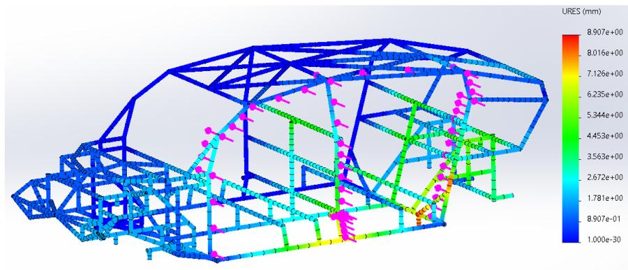
**Figure 8.** Simulation Results of Side Impact Static Test
