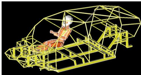
**Figure 1.** Demonstrate the positioning of the driver to align with the main structure
