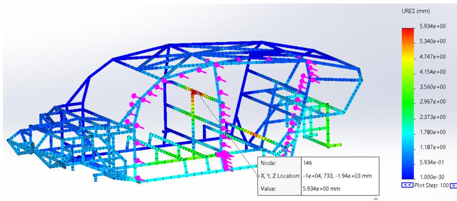
**Figure 9.** Simulation Results of Side Impact Dynamic Test at Node 146
