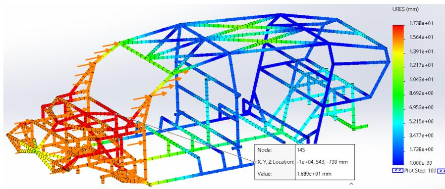
**Figure 6.** Simulation Results of Front Impact Dynamic Test at Node 145
