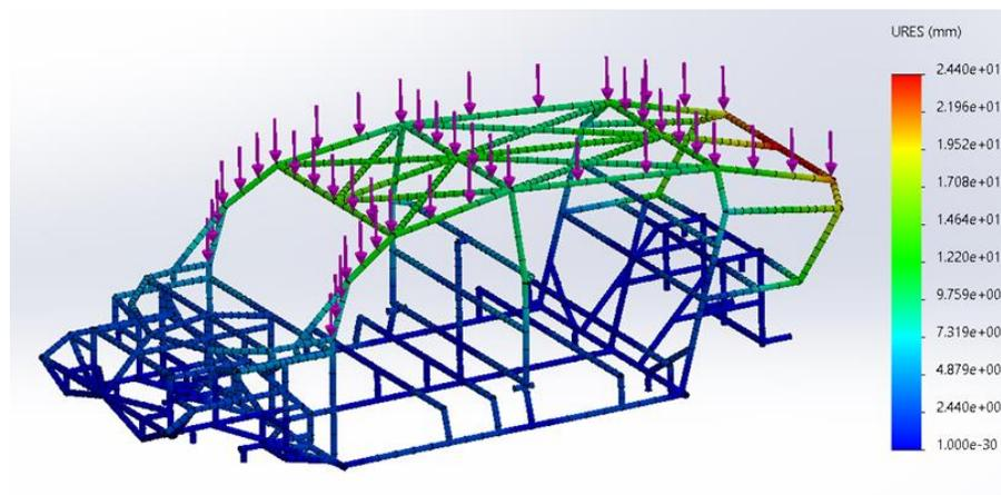
**Figure 2.** Simulation Results of Top Impact in Static Test
