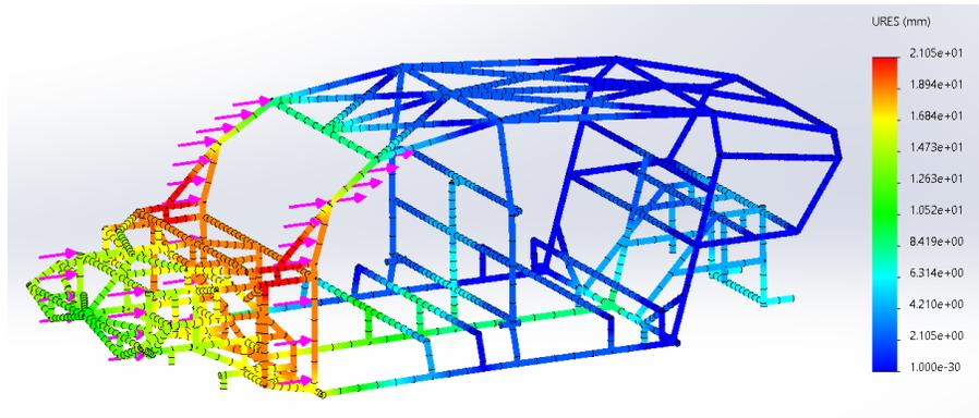
**Figure 5.** Simulation Results of Front Impact Static Test
