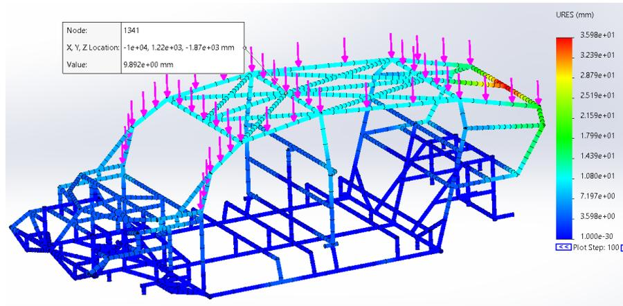
**Figure 3.** Simulation Results of Top Impact Dynamic Test at Node 1341
