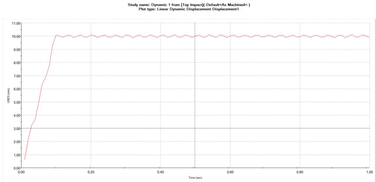
**Figure 4.** Dynamic Crush Analysis at Node 1341
