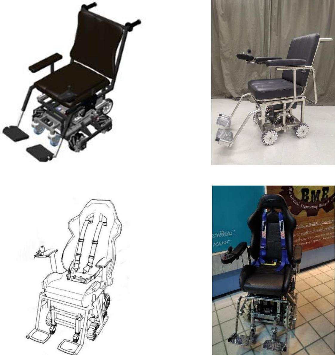
**Figure 2.** Electric cart controlled by mecanum wheels
