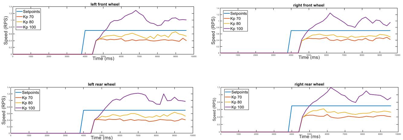
Figure 7. System response of a Mecanum Wheelchair employing P control
