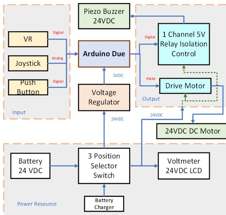
**Figure 1.** Schematic diagram of the electric cart control system
