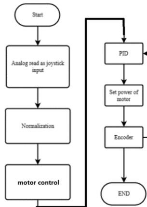
**Figure 4.** The workflow of system operation
