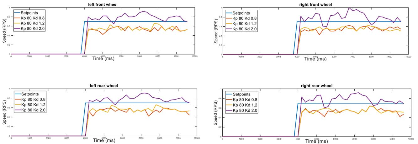
Figure 8. System response of a Mecanum Wheelchair employing PD control
