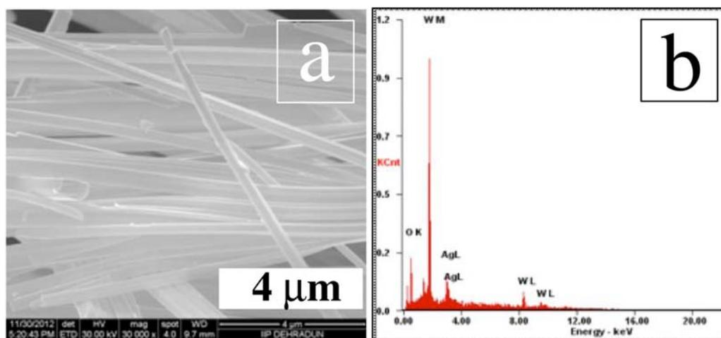
**Figure 2:** (a) SEM image and (b) SEM-EDAX image of Ag/WO<sub>3</sub> catalyst.
