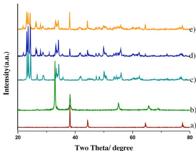
**Figure 1:** XRD patterns of **a)** Ag (0), **b)** Ag (I) oxide, **c)** W(VI) Oxide, **d)** prepared Ag/WO<sub>3</sub> catalyst **e)** spent Ag/WO<sub>3</sub>.
