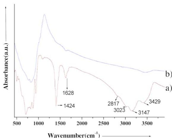
**Figure 4:** FT-IR of the **a)** uncalcined Ag/WO<sub>3</sub> catalyst and **b)** calcined Ag/WO<sub>3</sub> catalyst.
