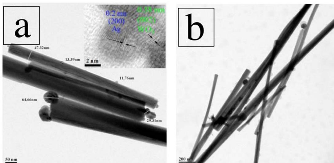
**Figure.3:** (a) TEM image of the fresh catalyst, inset lattice fringes, and (b) TEM image of the spent (after 3 recycles) Ag/WO<sub>3</sub> catalyst.
